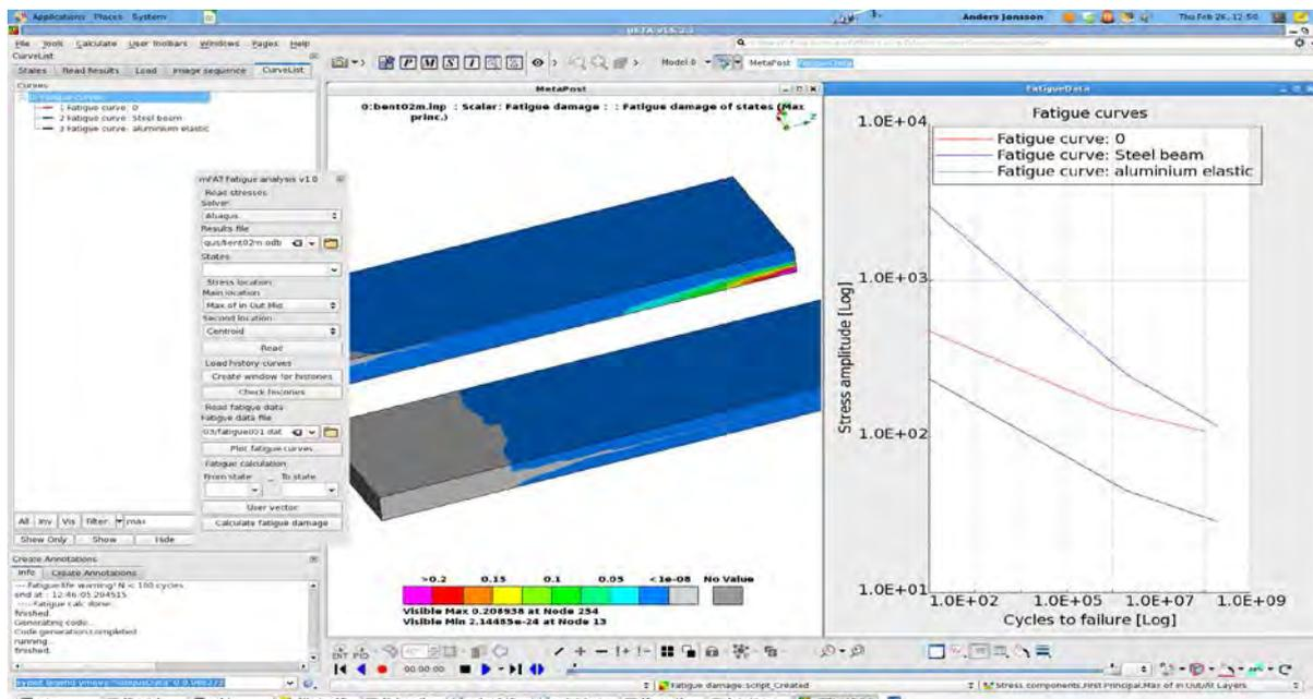
Figure 1. The mFAT fatigue post-processing module.
