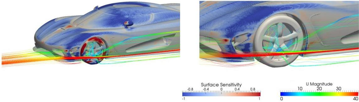
**Figure 15** Velocity-coloured Streamlines superimposed on Surface Sensitivity  $G_w$
