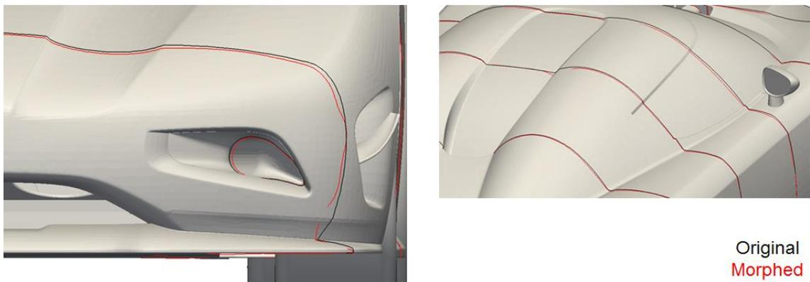
**Figure 17** Comparison of original to morphed geometry
