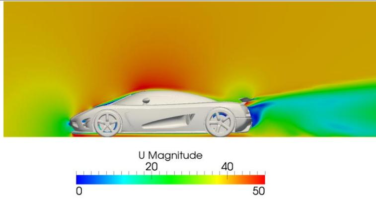
**Figure 9** Velocity Magnitude, section on  $Y=0$
