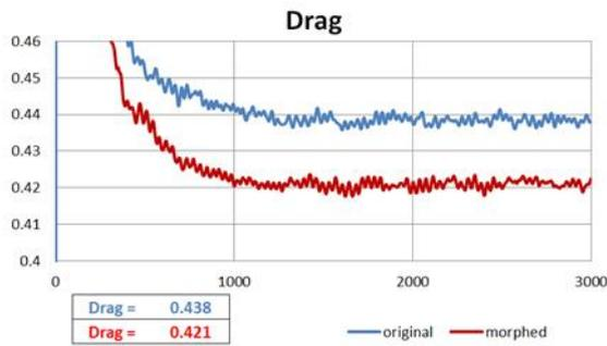
Figure 19 Drag (original & morphed geometry)
