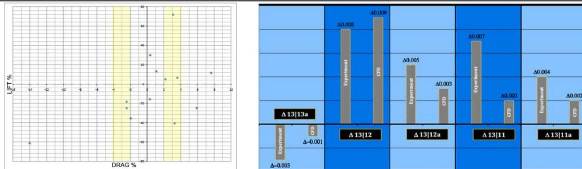
**Figure 6** Drag & lift CFD value prediction compared to experiment
