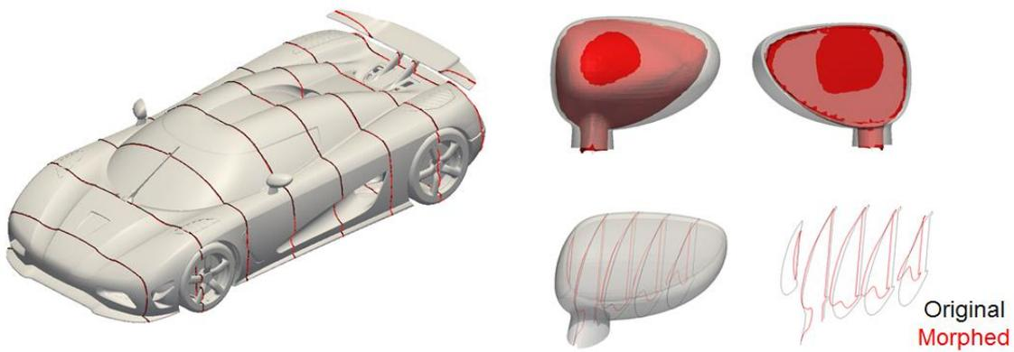
**Figure 16** Comparison of original to morphed geometry
