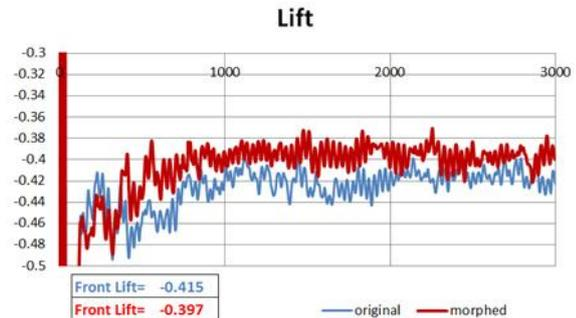
Figure 20 Lift (original & morphed geometry)
