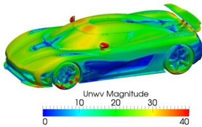
**Figure 10** Near Wall Velocity Magnitude  $Unwv$
