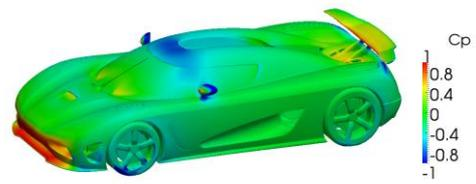
**Figure 11** Pressure coefficient
